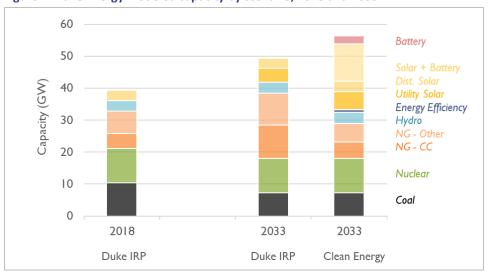
Figure 1. Duke Energy modeled capacity by scenario, 2018 and 2033
