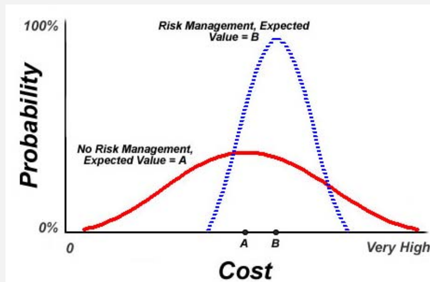
Figure 3.1. One view of the possible impact of hedging on risk exposure for the cost of a portfolio of resources.
