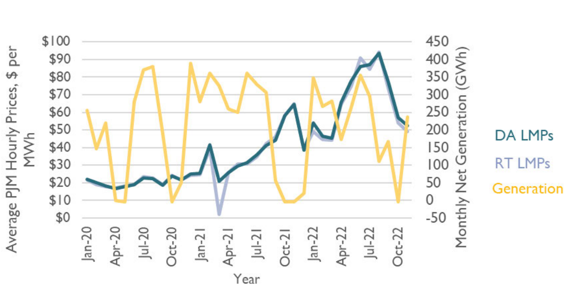
8 Figure 2. PJM hourly day-ahead (DA) and real-time (RT) locational marginal prices 9 (LMP) for the East Bend node, and East Bend generation
