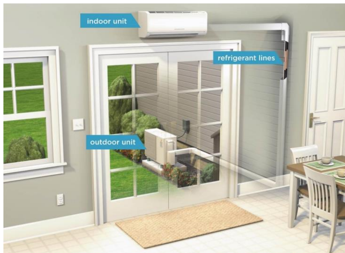
Figure 5. Ductless mini-split ASHPs use refrigerant pipes (instead of ducts) to deliver heating or cooling to each room where an indoor unit is installed.
