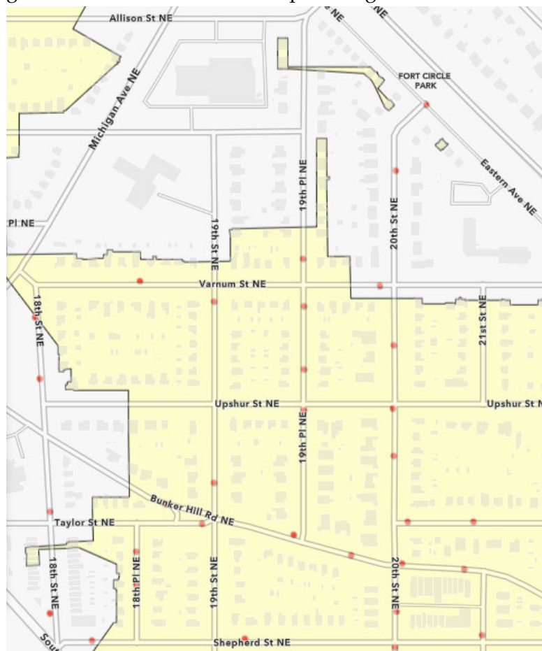
Figure 16. Woodridge focus area. K Street SE, was investigated in this study. Red dots indicate gas leaks detected in Phase 1 report; beige shaded areas indicated areas serviced with gas.
