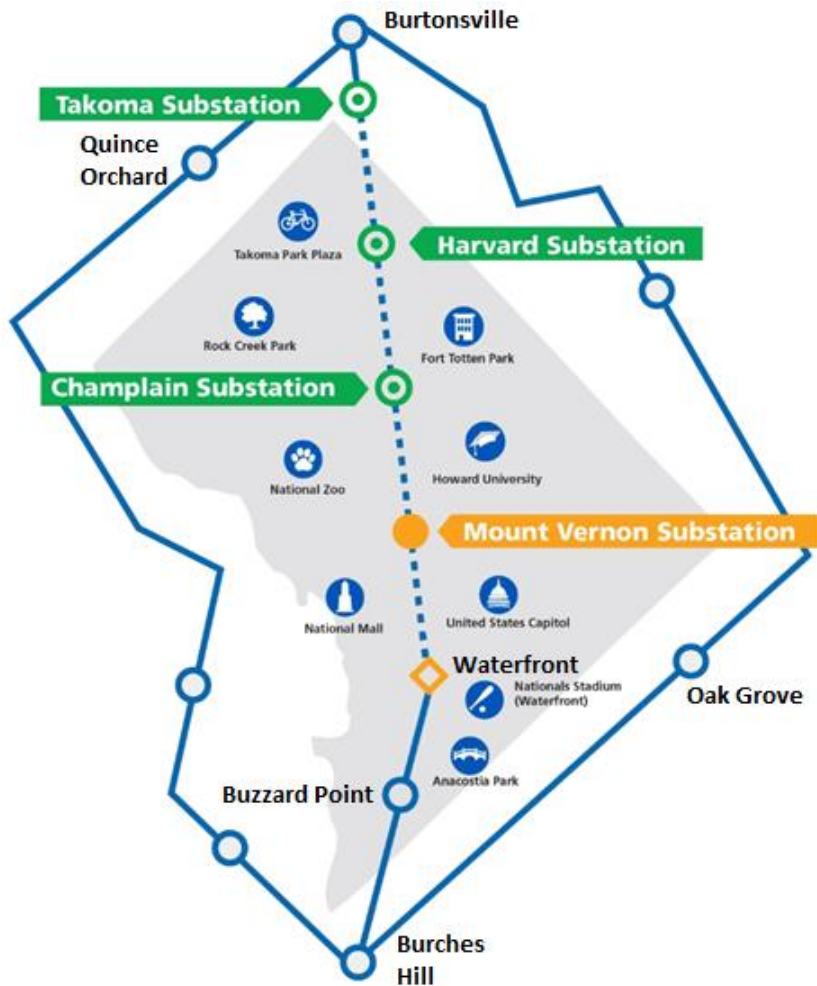
Figure 3. Annotated Pepco diagram showing the Capital Grid project: three upgraded substations (green), a new transmission line (dashed line), and the new Mt. Vernon Substation
