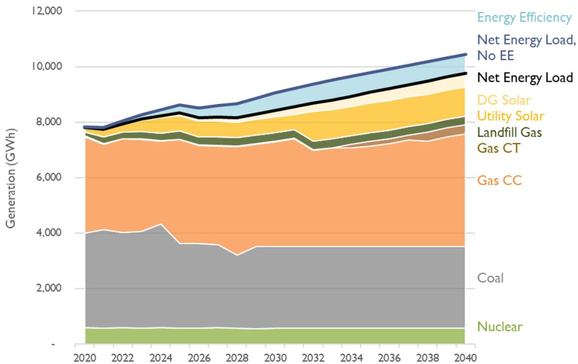
Figure 7: Coal to Gas Conversion—generation
