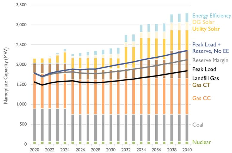
ES Figure 2: Coal to Gas Conversion—nameplate capacity
