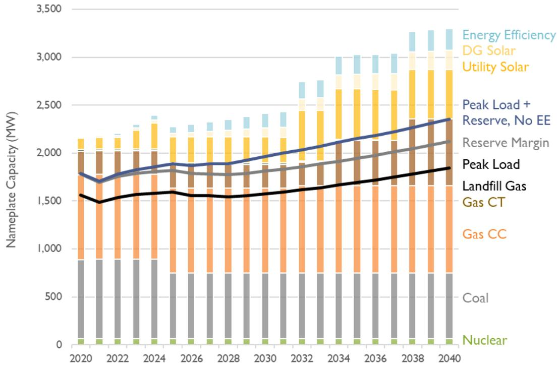
Figure 4: Nameplate installed capacity for *Coal to Gas Conversion* scenario
