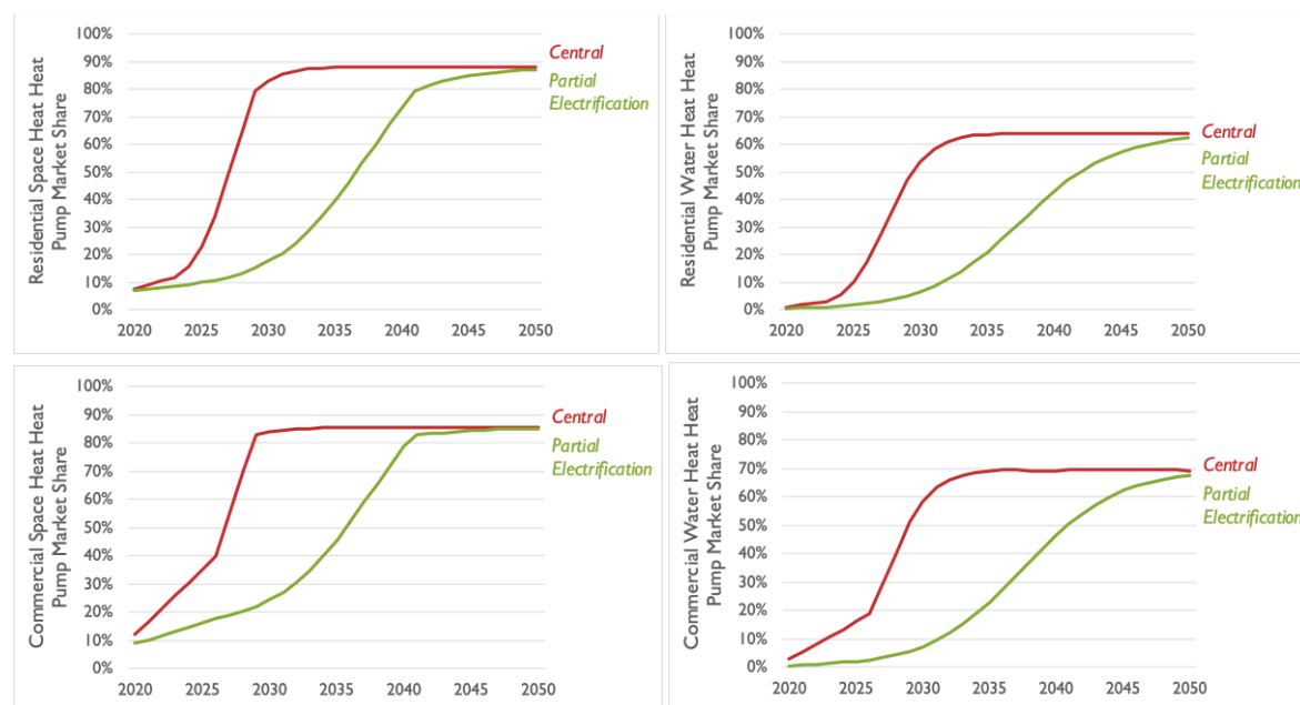
Figure 4.19 Heat pump market shares of new system sales in the Partial Electrification (green) and Central (red) scenarios through 2050. Results for residential buildings are on the top and results for commercial buildings are on the bottom. Results for space heating heat pumps are on the left and for water heating heat pumps are on the right.
