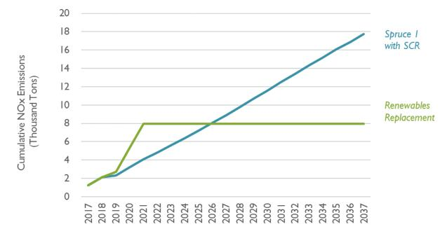
Figure 11. Cumulative Spruce Unit 1 NO<sub>X</sub> emissions under 2019 SCR retrofit vs. 2022 renewable replacement
