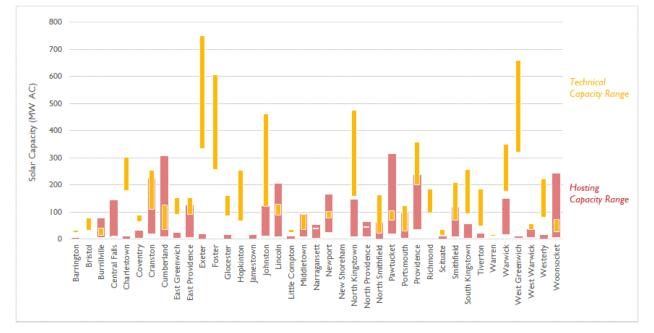
Figure 32. Technical solar capacity and hosting capacity ranges for each municipality in Rhode Island
