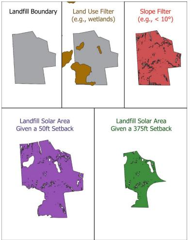
Figure 13. Schematic of the approach to calculating area for landfill solar technical potential
