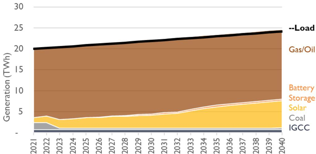
In the 50% Clean Energy Scenario, TECO’s load declines due to increased investment in EE and DSM. The Company continues to rely on gas in the early years but is able to displace a significant portion of its gas generation with solar PV over the next two decades. By 2035, over 9.5 TWh of load is served by solar generation. This amount would easily allow the City of Tampa to achieve its 100 percent renewable energy resolution.
