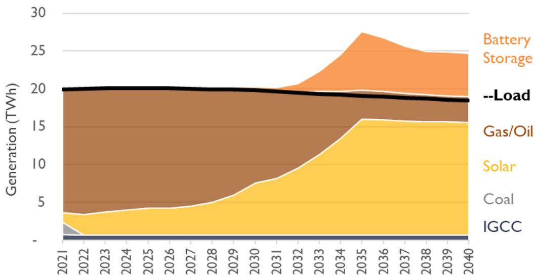
The generation results from the high gas and carbon price sensitivities also look quite similar to the results presented in Figure 7 through Figure 9. Because the resource mix is unchanged between the sensitivity and the original scenario, the model has limited dispatch flexibility.
