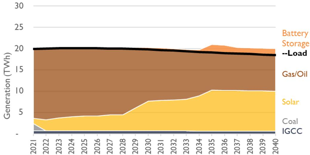
In the 80% Clean Energy Scenario, the generation is similar to the 50% Clean Energy Scenario up until 2030. After that, the model ramps up its solar production and utilizes battery storage to a higher degree. By 2035, solar generation amounts to over 15 TWh. This vastly surpasses the amount required for the City of Tampa to meet its 2035 target. The full generation results of this scenario are shown in Figure 9.
