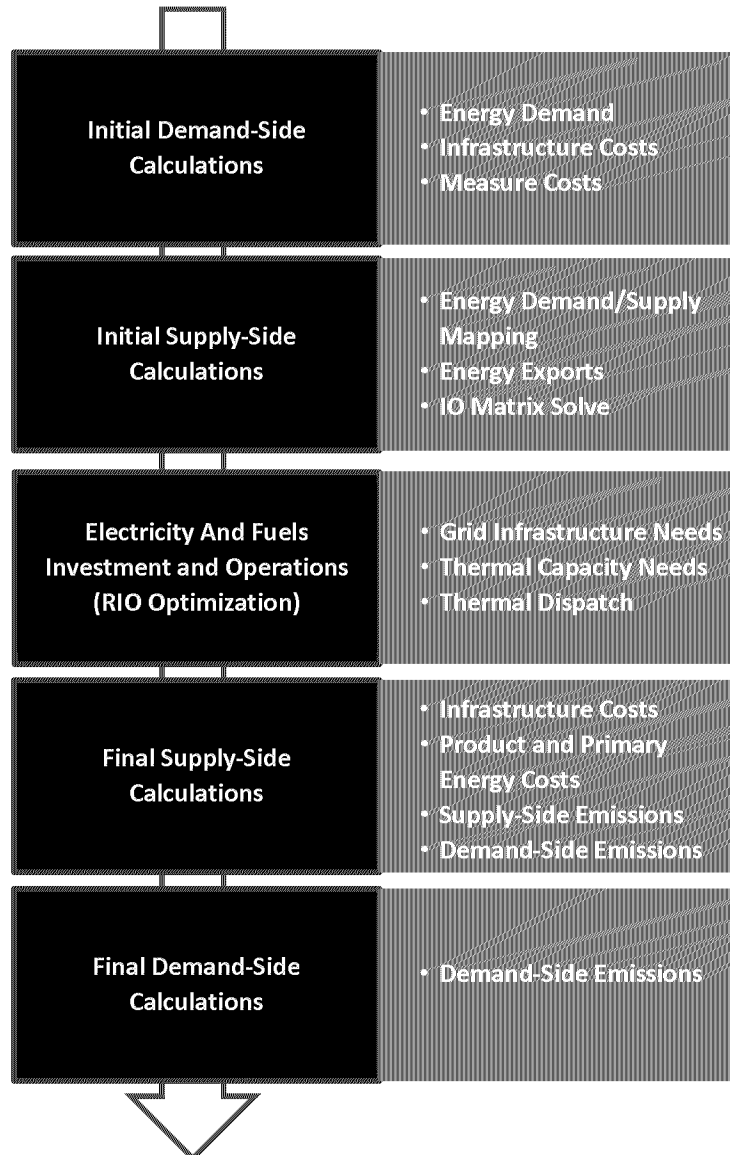
Figure 66 shows the basic calculation steps for EnergyPATHWAYS and the outputs from each step.
